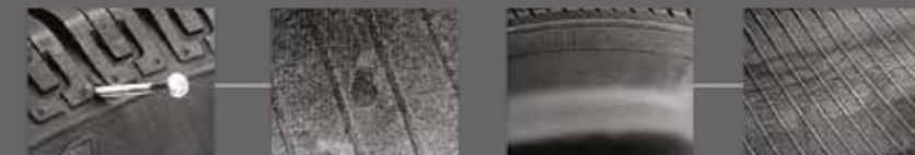
Puncture – Normally, the only evident of a puncture will be a cut that extends from the tread of the tire through the inner liner. Under-Inflated Tire – An abrasion may run around the circumference of the tire and wrinkles may be observed in the inner liner.
